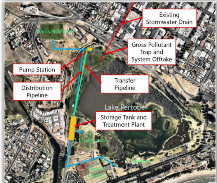
Figure 13: Excerpt from Lake Pertobe Master Plan 2018 showing schematic of a potential stormwater irrigation scheme
