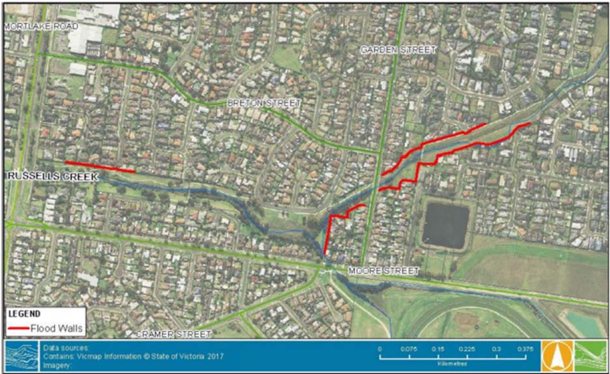
Figure 2. Location of the constructed flood walls. (Source; Water Technology 2017).
