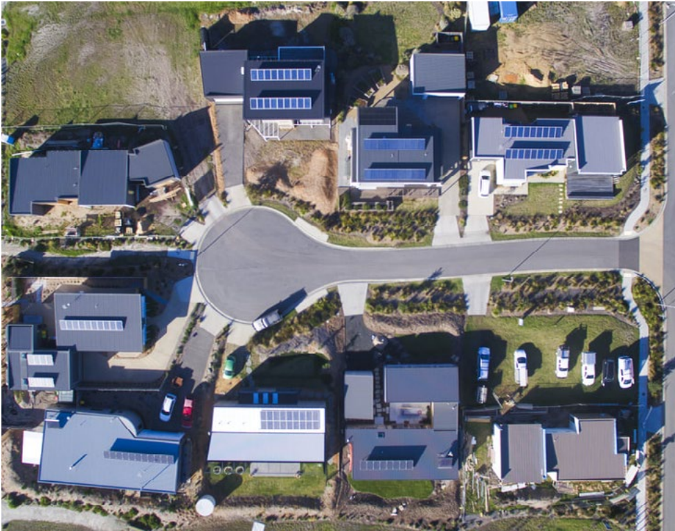
IMAGE: EACH DWELLING AT THE CAPE IS EQUIPPED WITH MINIMUM 2.5KW ROOFTOP SOLAR PV SYSTEM (SOURCE: LIVINGATTHECAPE.COM)
