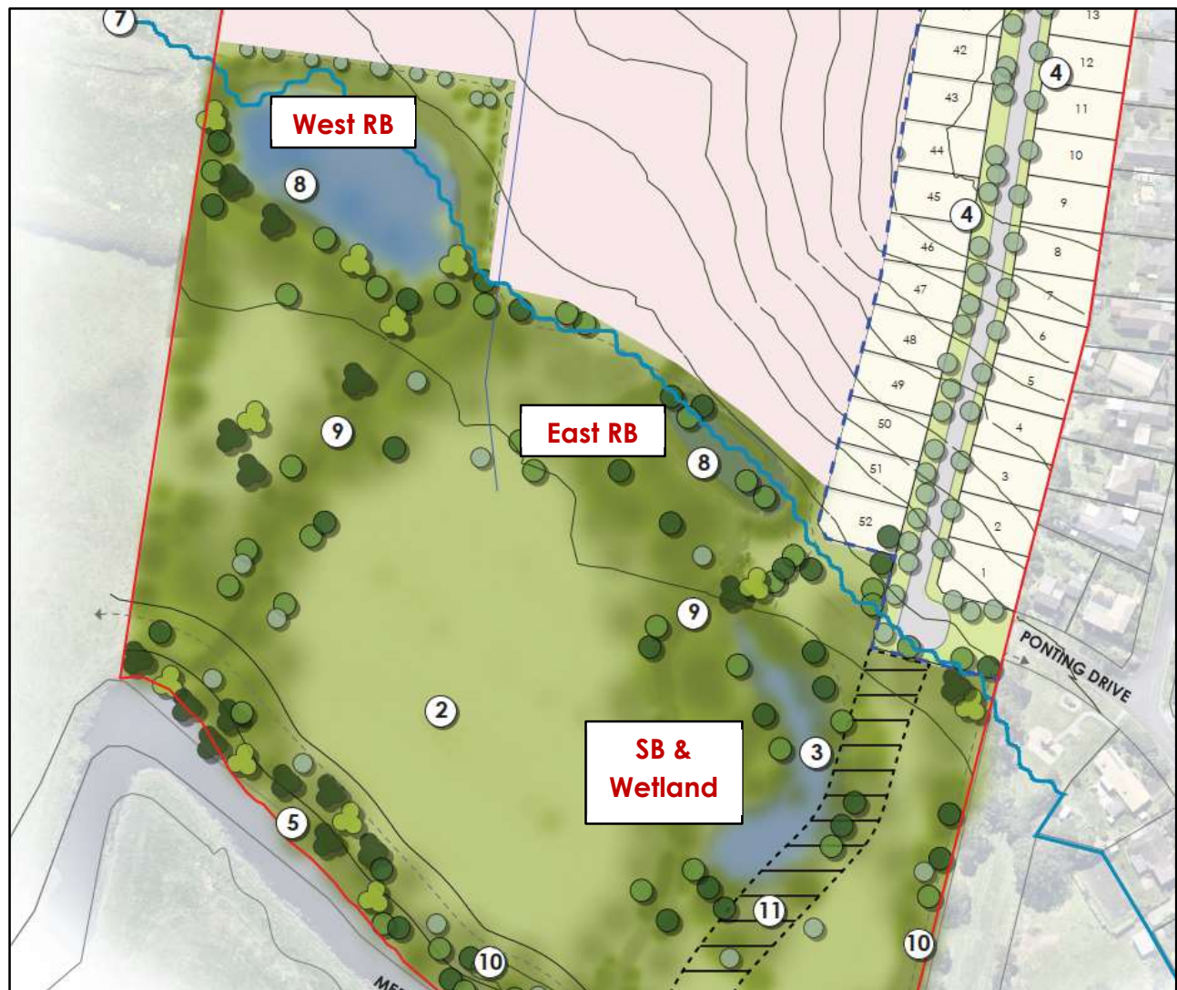
Figure 5: Drainage Assets Location Plan
