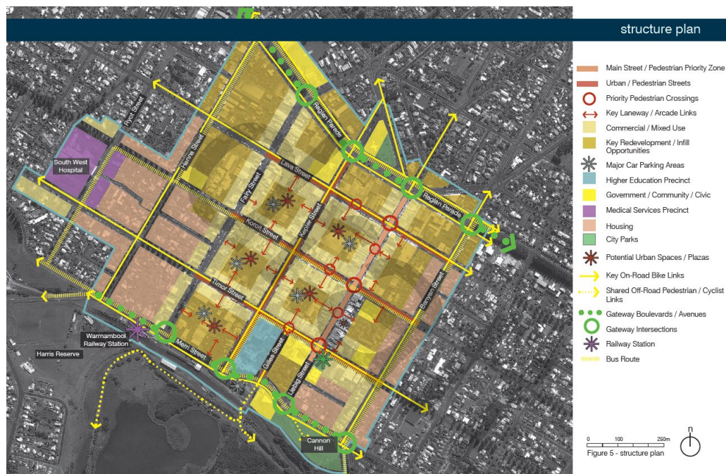
Figure 1: Warrnambool City Centre Revitalisation Structure Plan 2012
