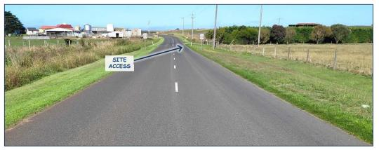
Council traffic data (2013 & 2015) sets out that Tooram Road carries a daily traffic volume in the order of 600 vehicle movements per day, with 14% trucks. Recorded 85<sup>th</sup> percentile speeds between Hermitage Drive and Morgans Road were 94kph and 95kph within a 100kph speed zone.
