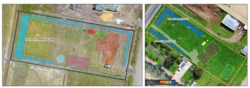
Figures 12-13 - Utilisation of cross-contour pressurised subsurface irrigation to tussock and sedge-dominated indigenous plantings.
