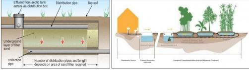
Figures 25-26 – Sand Filter System components; Rhizopod system supporting upgrade options on small lots where the Rhizopods are added post-septic tank to reduce effluent disposal area required (Source: Arris Wastewater Technologies 2019). (Source: Golden Plains Shire Council 2015, EPA 2016).
