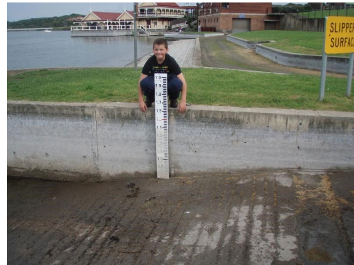
Figure 26. Simpson Street boat ramp water level monitoring board
