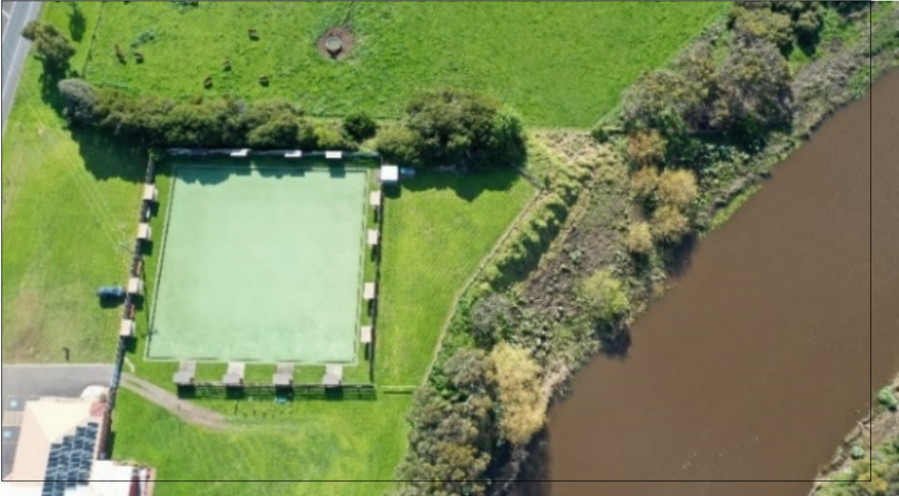
Figure 45- High-risk effluent disposal adjoining (within 30m setback) the Merri River. Excessive weed growth within adjoining parts of the river provide a clue to this system's sustainability and reason to connect to sewer.
