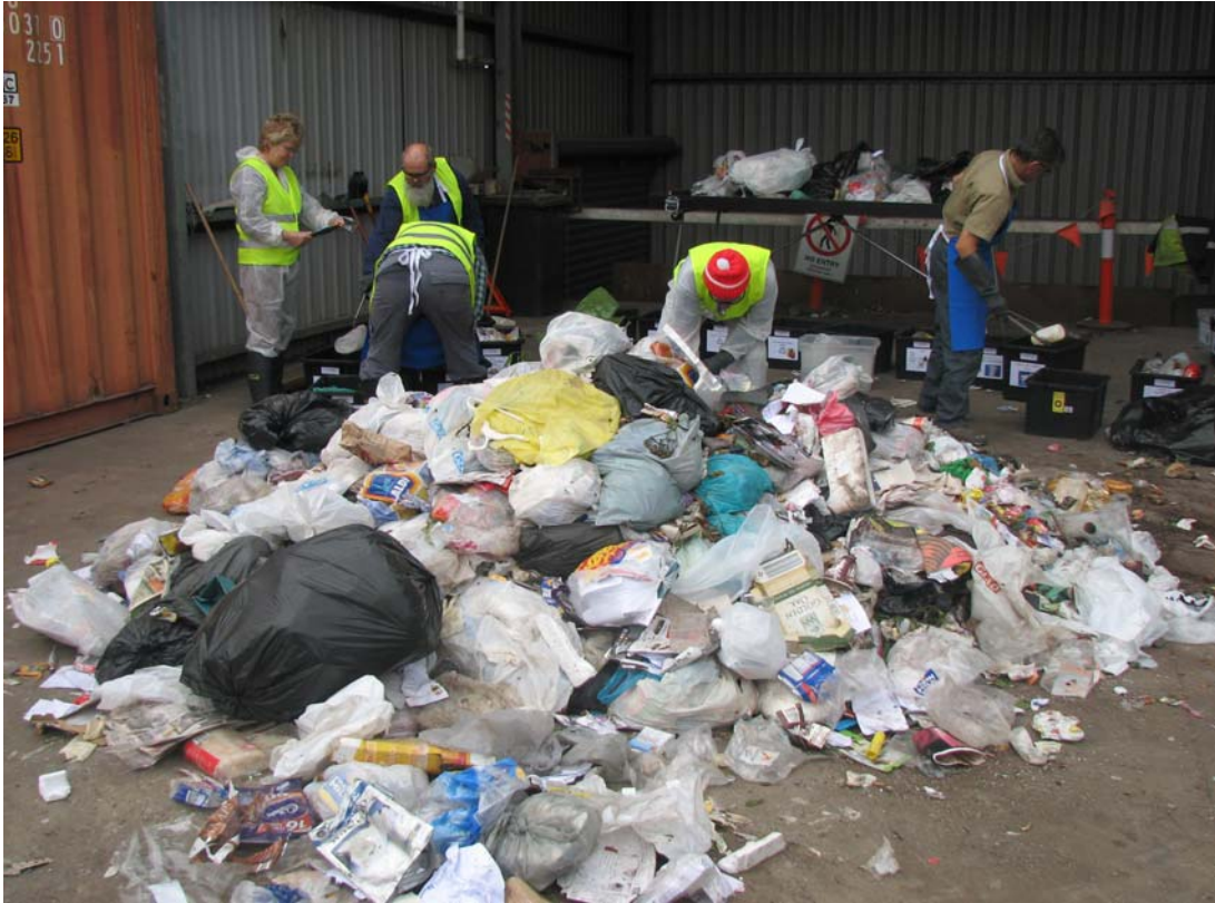
Bags of waste were transferred to a sorting table, tongs were used to separate the waste into the different waste streams.
