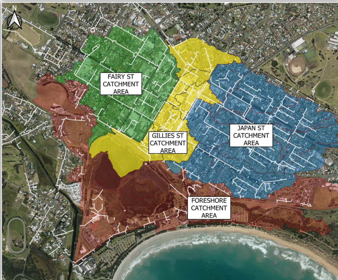
Figure 3: Stormwater catchments flowing into Lake Pertobe (small white lines indicate the stormwater pipe network)
