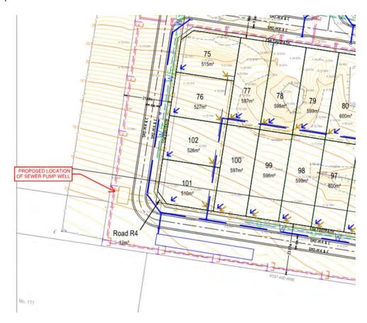
Figure 2: Proposed location of sewer pump well
