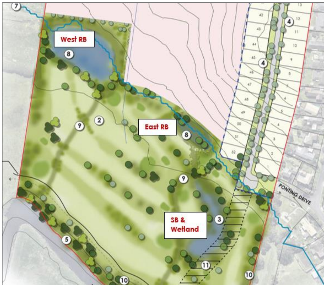
Figure 5: Drainage Assets Location Plan
