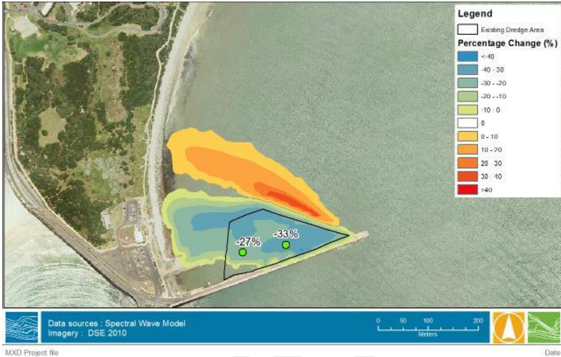
FIGURE 2-20 PREDICTED PERCENTAGE CHANGE IN SIGNIFICANT WAVE HEIGHT BETWEEN THE PRE (2011) AND POST (2013) MAINTENANCE DREDGE SIMULATIONS. (WATER TECHNOLOGY, 2013)
