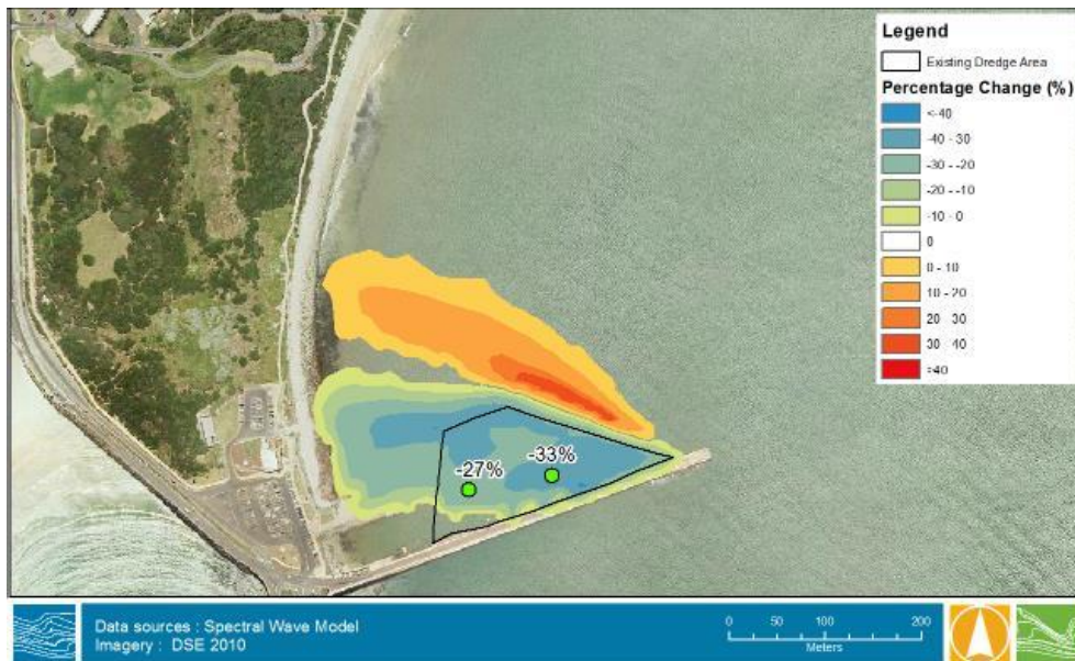
FIGURE 2-4 PERCENTAGE CHANGE IN SIGNIFICANT WAVE HEIGHTS FROM PRE- AND POST-DREDGING
