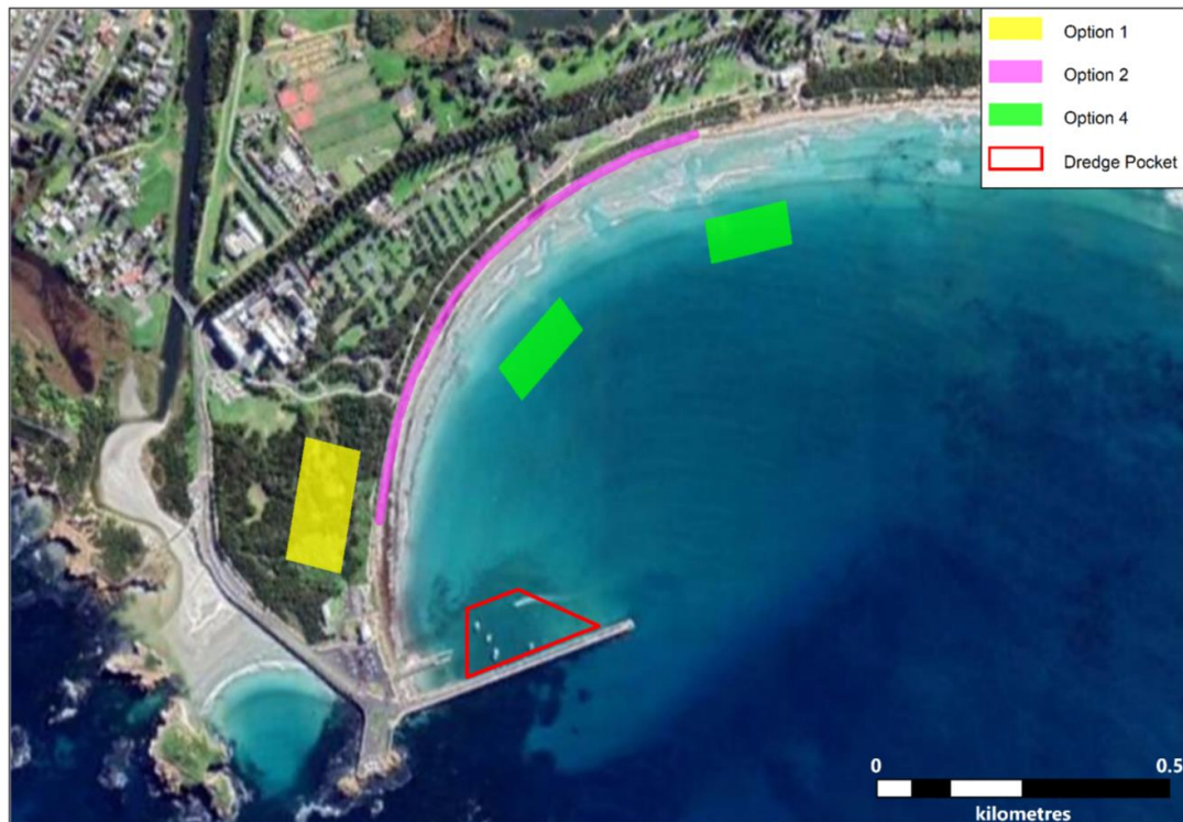
FIGURE 4-1 DREDGE SAND REUSE OPTIONS
