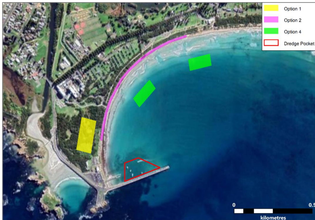
FIGURE 4-1 DREDGE SAND REUSE OPTIONS
