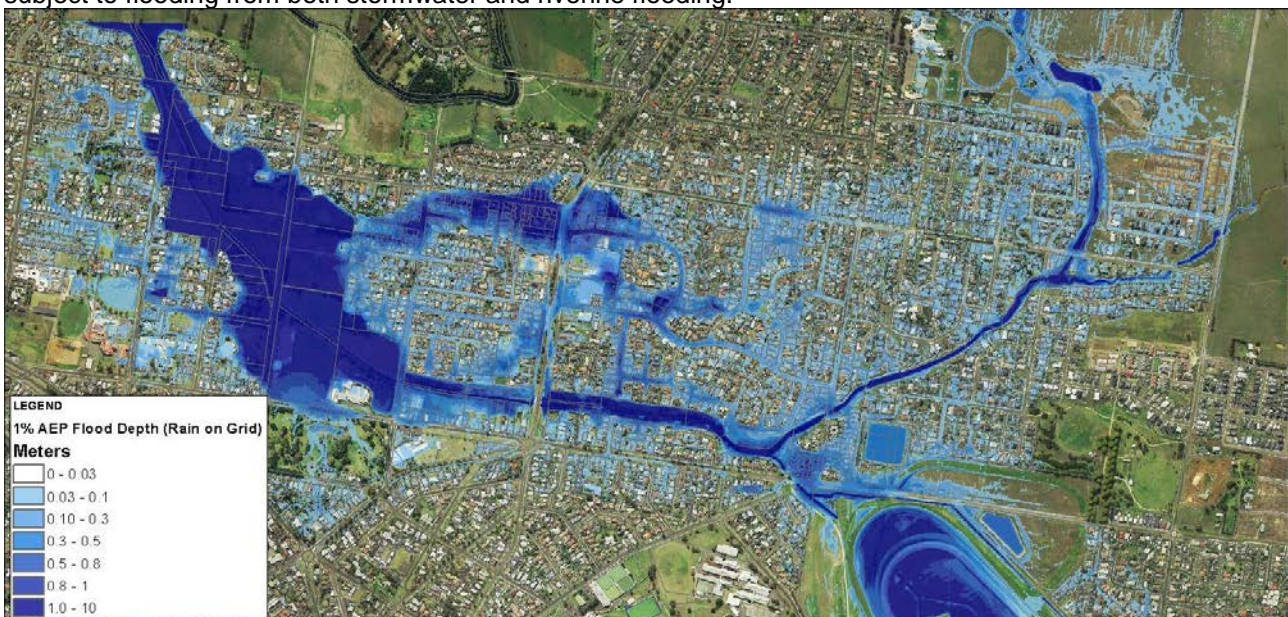
Figure: 1% AEP Rain on Grid (sensitivity testing)
