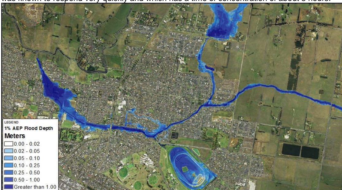
Figure: 1% AEP Flood Depth (New Existing Conditions)
