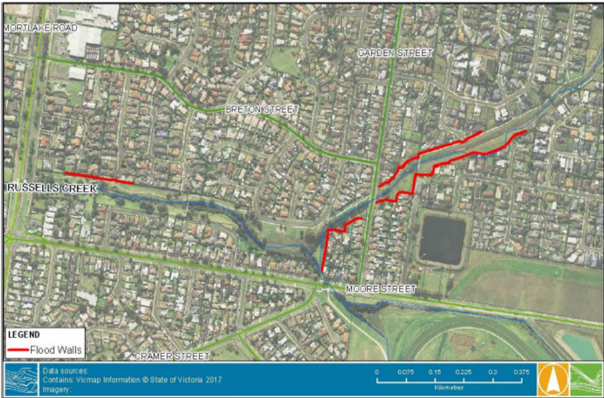
Figure 2. Location of the constructed flood walls. (Source; Water Technology 2017).
