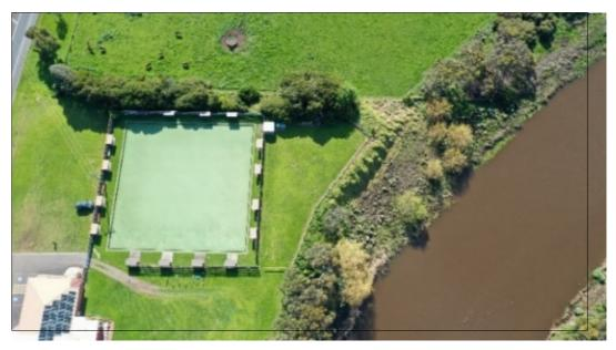
Figure 45- High-risk effluent disposal adjoining (within 30m setback) the Merri River. Excessive weed growth within adjoining parts of the river provide a clue to this system's sustainability and reason to connect to sewer
